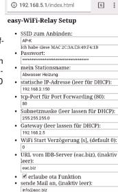
· lokale Watchdog http-IP (192.168.1.1), (inaktiv leer): · matt Port, default 1883: mqtt send cycle [0-43200s], default 20: mqtt topic (S25/KG/eWR) S25/KG/eWR · Info: Rohrheizung Abwasser KG ?sw=0 heizt nc closed speichern | verlasse Setup | neu laden easy-WiFi-Relay: Abwasser Heizung Switch no : closed --> OPEN Switch nc Pulse 10s MOTT connected: 1, sr 12, recomment 0, sels 100 Heartbeat hb : 4 min ping Monitor m3-08c000, vom Jan 25 2019 10:29:26
